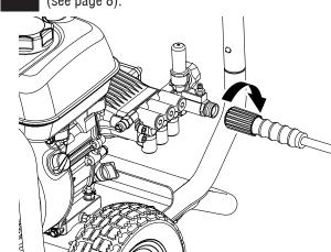
Completely uncoil and straighten high pressure nose to prevent kinks.
