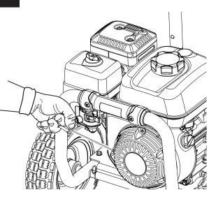
Allow engine to run for several seconds, then move choke to OFF (RUN) position (see page 10).
